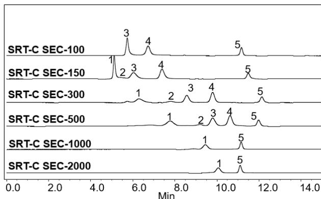
Figure 1. Elution profiles of a protein mixture by SRT-C SEC-100, SRT-C SEC-150, SRT-C SEC-300, SRT-C SEC-500, SRT-C SEC-1000, and SRT-C SEC-2000 columns: 5 $\mu\text{m}$ , 7.8x300mm; Mobile phase: 150 mM Sodium Phosphate buffer, pH 7.0; Flow rate: 1.0 mL/min; Detection: UV 214 nm; Temperature: ambient (23  $^{\circ}\text{C}$ ); Injection volume: 5  $\mu\text{L}$ .
